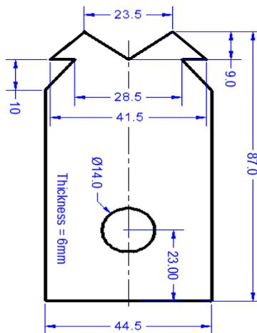
Figure 5. The sizes of the designed hammer
