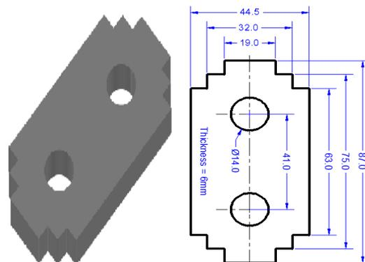
Figure 2 – (a) The size of the conventional hammer –
