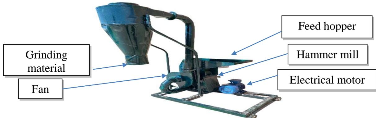
Figure 1. The main parts of the investigated hammer mill
