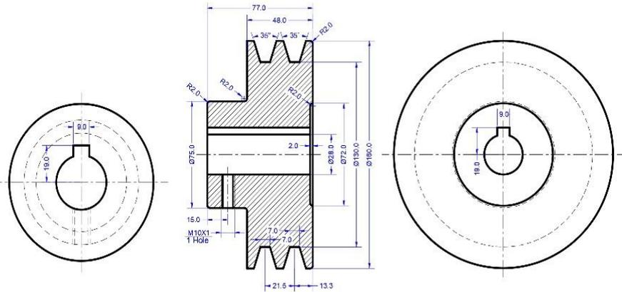
Figure 4. The sizes of 16 mm pulley
