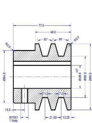
Figure 3. The sizes of 8 mm pulley
